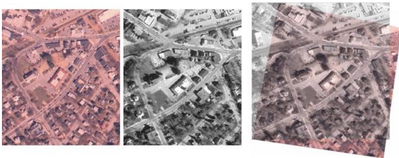
Image registration on satellite imagery [Sommervold et al., 2023]
