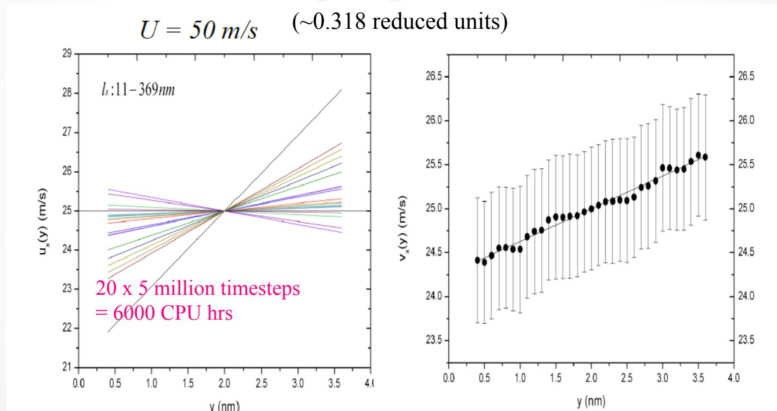
Couette:  $\text{H}_2\text{O}$ ,  $L_s$  (EMD) =  $60 \pm 6 \text{ nm}$ ; NEMD =  $61 \text{ nm}$
