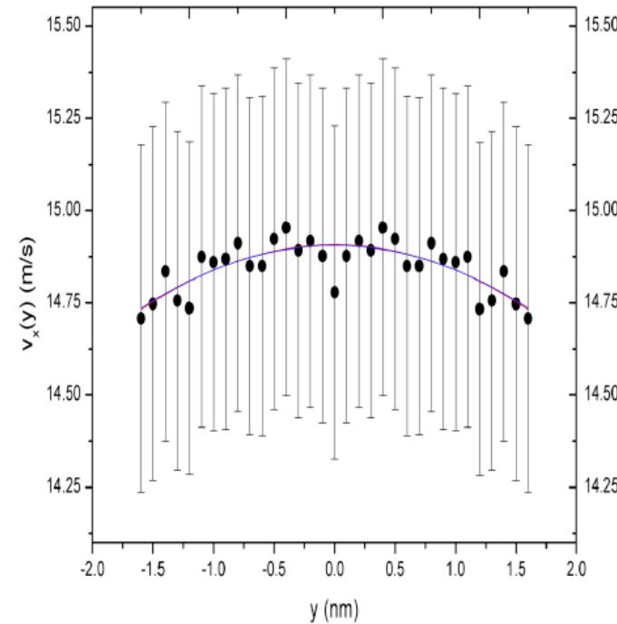
Poiseuille:  $\text{H}_2\text{O}$ ,  $L_s$  (EMD) =  $60 \pm 6$  nm; NEMD = 53 nm
