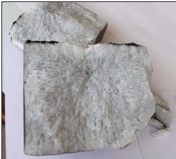
Salt ingot obtained after rapid solidification
