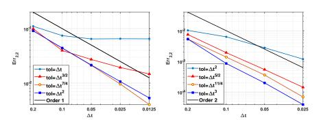
Figure: Comparison of the order of convergence for the pruned TSA with different tolerances (left) with Euler method and (right) with Heun's method.
