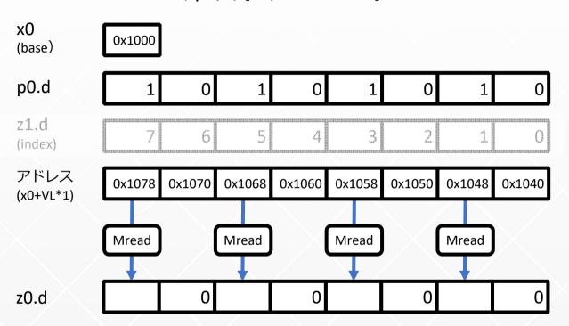
VL is 64 in byte when vector length is 512bits.
