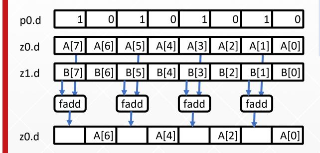
This example uses "double precision". There are other types; "single precision", "half precision", integer (64bit, 32bit, 16bit, 8bit)
