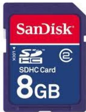
**Flash memory** is a non-volatile computer storage chip that can be electrically erased and reprogrammed.
