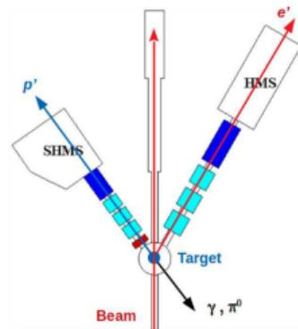
(d) Experimental configuration for  $\text{tH}(e', ep)\pi^0$  with the standard Hall C equipment
