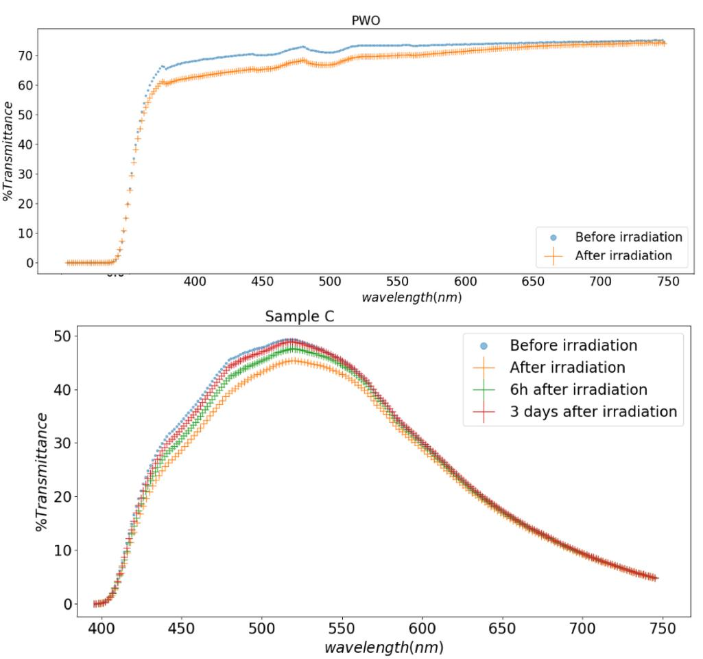
Transmittance measurement to assess the creation of light-absorbing centers with radiation damage.
